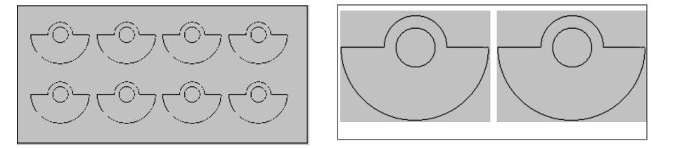
More vibrating weight Less amplitude Less vibrating weight More amplitude
