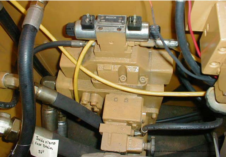
Control panel showing how power cables for solenoids can be removed quickly.
