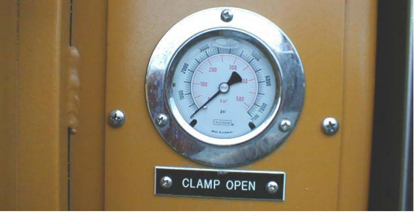
Clamp open reads the actual relief valve setting on the clamp manifold. You are reading the safety relief valve setting.Note: This is not the valve you change if you are wishing to lower pressure on the clamp. Use the pressure switch for that. This gauge reads your pressure setting and it should be at
