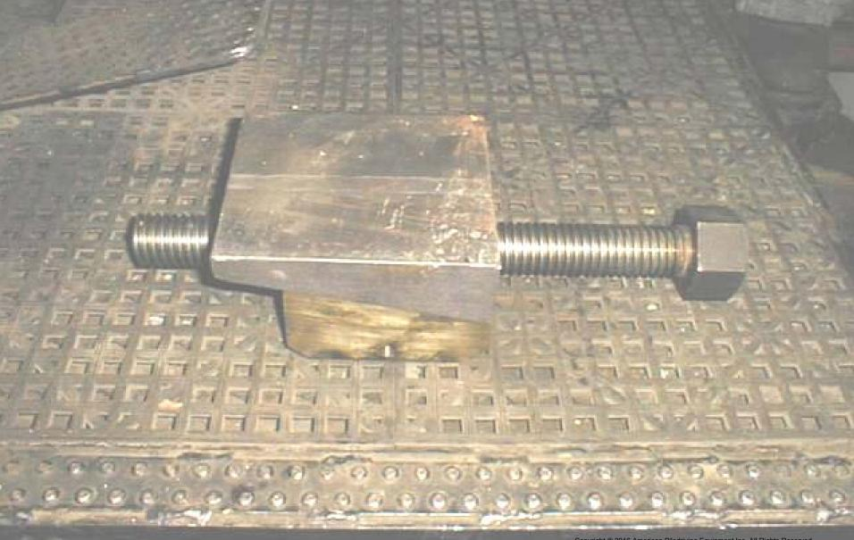
Wedges must be greased. If wedges are not tight the vibro will not put energy into the casing.
