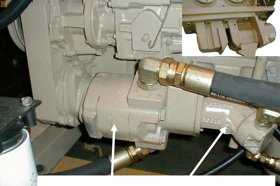
Cooling pump with piggy back clamp pump.
