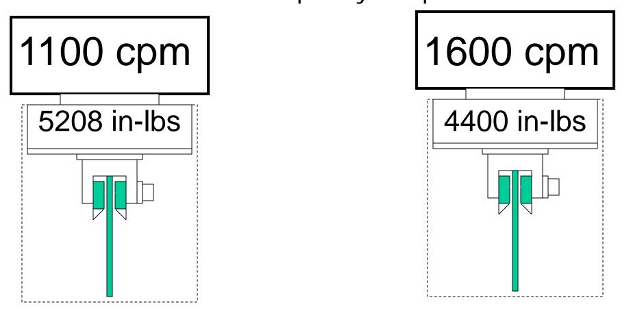
$\frac{5208 \times 0.0142 \times 1100 \times 1100}{1,000,000} = 89 \text{ tons} \quad 159.94 = \frac{4400 \times 0.0142 \times 1600 \times 1600}{1,000,000}$
